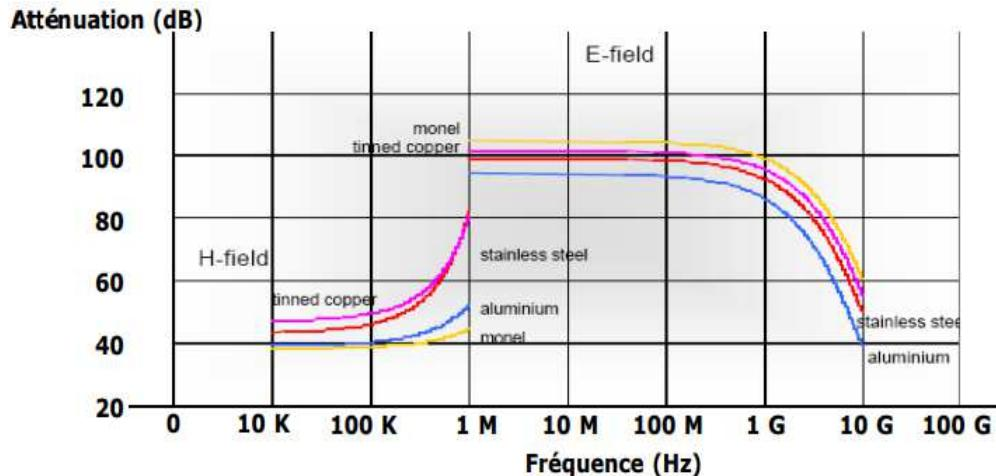
This graph compares the overall performance of our joints in fields E and H, manufactured with different materials: monel, stainless steel, tinned copper and aluminum. The test results presented here are made with cellular silicone type D05 and 2 layers of knitting according to MIL STD 285.
